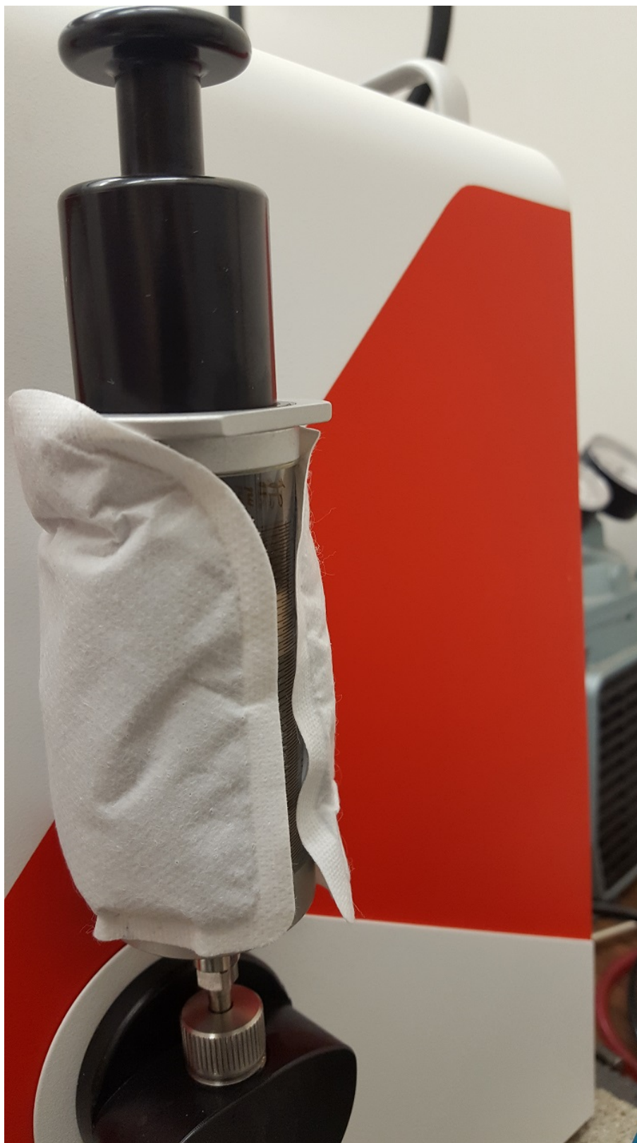
Figure 1. A toe warmer wrapped around a syringe that is mounted to the Eralytics instrument.
