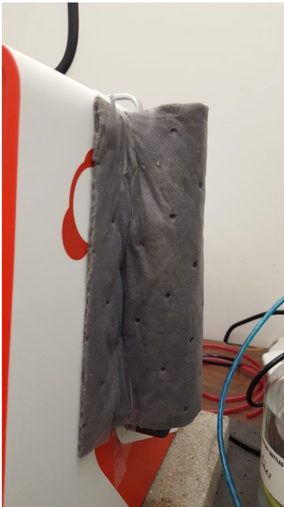
Figure 2. Insulation around a syringe that is mounted to the Eralytics instrument.
